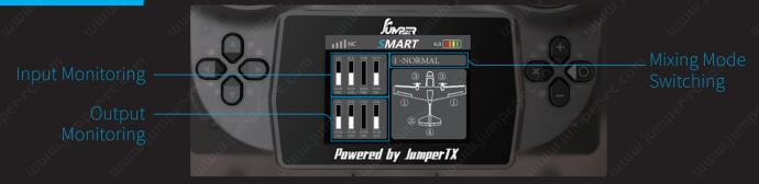
3. Press and hold the "O" button to enter the mixing settings. Use the left-side directional buttons (Up, Down, Left, Right) to set the direction (normal/reversed) and travel range for CH1-CH4. Press the "O" button again to toggle between normal and reversed direction. Use the "+" and "-" buttons to adjust the travel range. The "×" button exits.
