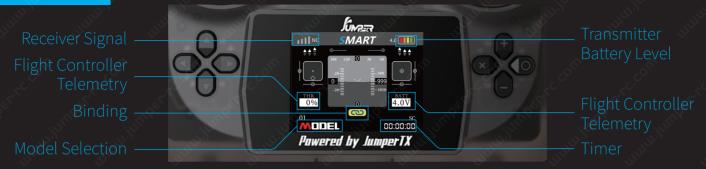
Press and hold the "O" button to enter the menu. Use the left-side directional buttons (Up, Down, Left, Right) to navigate through
