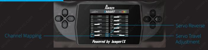
2. Press and hold the "O" button to enter the travel adjustment settings. Press the "O" button again to toggle between normal and reversed direction. Use the "+" and "-" buttons to adjust the travel range. The "×" button exits.
