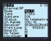
Status: Display the status of the multi-protocol module. (Normally it shows the firmware version of the multi-protocol module)
