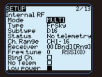
Status:Display the status of the multi-protocol module. (Normally it shows the firmware version of the multi-protocol module)
