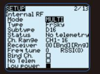
**Freqtune**: Frequency tuning. Certain protocols require tuning for optimal performance. In some cases, tuning is required in order for the protocol to bind. Frequency Tuning is specific to each MULTI-Module, and is due to very small variations in the RF components.
