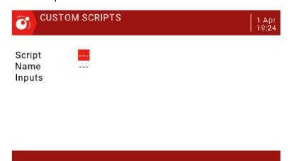
You can select a script in the first line and optionally define a custom name to know what to use in the second line. The screen also displays the inputs and outputs used by the script.
