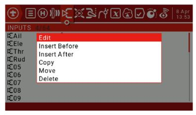
Move the cursor to Ail, press and hold ENT to enter the edit pop-up window, then select the Edit option and press ENT. We use a 15% Expo curve to ease the response
