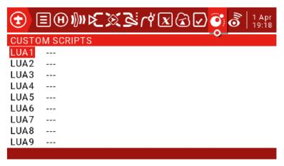
The Custom Scripts page is used for mixed-type scripts that run continuously. These scripts should be placed in the SD card / SCRIPTS / MIXES / folder.
